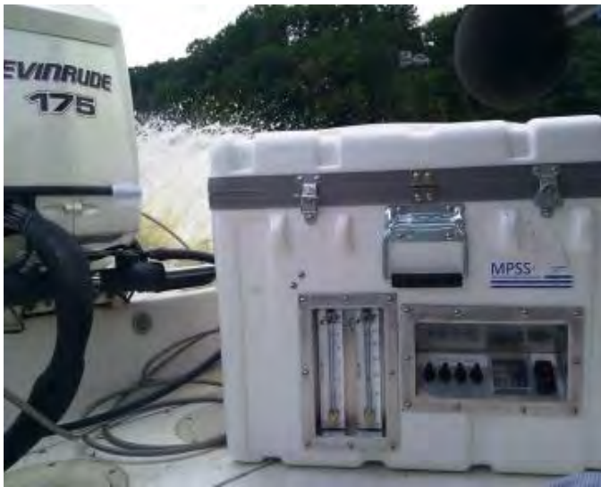
Figure 4. MPSS Bag Sampling System in use in the 18' Mako boat
