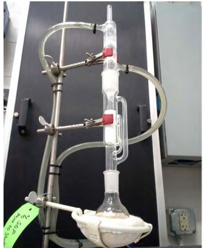
Figure 5. Soxhlet extraction using methylene chloride
