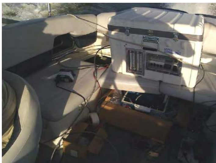
SeaDoo Challenger Jet-boat on water emissions evaluation Rotax 1503 Supercharged Four-stroke engine test set-up
