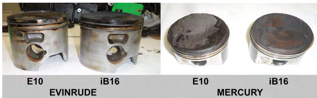
FIGURE 3. Comparison of Pistons (cylinder number 1) for the Evinrude and Mercury Engines Operated on E10 and iB16
