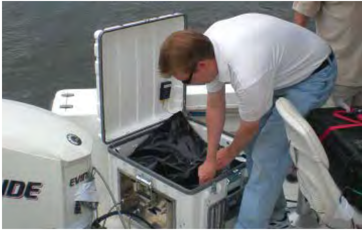
Evinrude engineer Jeff Wasil loads a fresh emissions-trapping pouch into the Marine Portable Sampling System (MPSS) that he designed.
