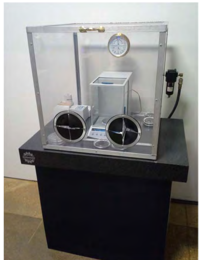
Figure 3. Constant temperature/constant humidity glove box - the scale sits atop a granite seismic mass table.
