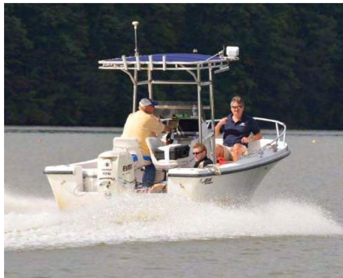
Figure 1. 18 foot Mako boat with 175 HP Evinrude Direct Fuel Injection Outboard undergoing on-water field emissions testing
