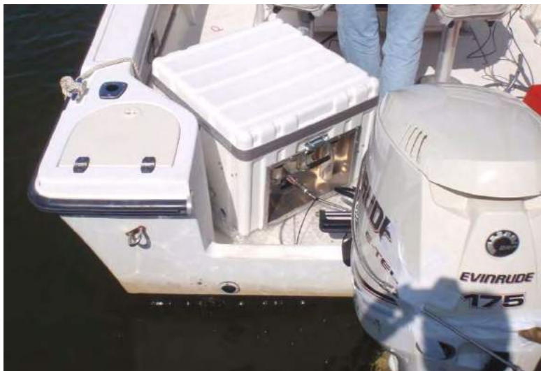
Evinrude E-TEC 175 Stratified Charged Direct Fuel Injection Two-Stroke on water emissions evaluation – 21' Mako Boat Test Set-up
